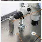
Integrated light source with heated glass
